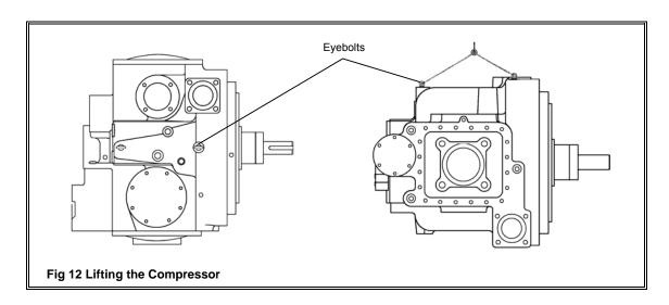
Check that the compressor mounting points on the baseframe are completely free from rust, dirt or burrs. Lift the compressor and make the same check at the compressor's three mounting points; check the tapped holes are undamaged and the threads are completely free of dirt.
