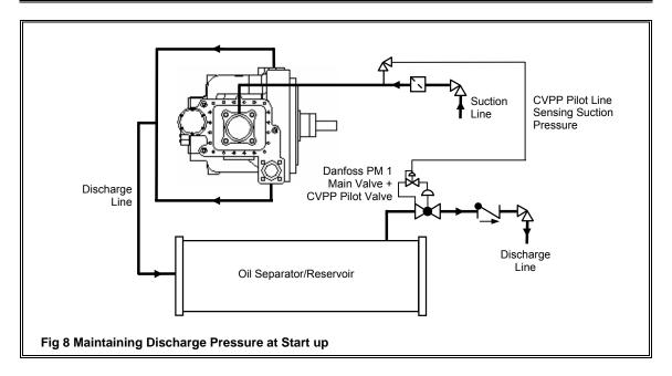
Discharge pressure, inlet pressure to the main valve, is applied to the space below the pilot valve diaphragm. Suction pressure is applied via a pilot line to the space above the diaphragm. The main valve, therefore, controls on the differential between suction and discharge pressure.
