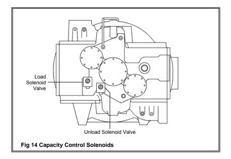
The solenoids must be connected to a suitable plant controller that will energise the appropriate coil to load or unload the compressor via changes to the operation of the system into which the compressor is fitted. The measured variable may be chilled water temperature, suction gauge pressure, etc.
